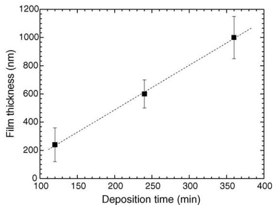
Fig. 4. Film thickness vs. deposition time for chromium (III, IV) oxides films processed with the following parameters:  $P_{\text{T}} = 50$  Pa,  $\Phi_{\text{Cr}} = 1$  sccm,  $\Phi_{\text{O}_2} = 1$  sccm,  $\Phi_{\text{Ar}} = 50$  sccm and  $F = 75$  mJ cm<sup>-2</sup>. (■), Experimental data; (- -), curve fit.
