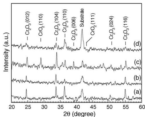
Fig. 2. XRD patterns of films deposited during 4 h at total pressure of 50 Pa,  $F = 75$  mJ cm<sup>-2</sup> and various  $p_{\text{O}_2}/p_{\text{Cr}}$  ratios: (a)  $p_{\text{O}_2}/p_{\text{Cr}} = 0$ ; (b)  $p_{\text{O}_2}/p_{\text{Cr}} = 0.7$ ; (c)  $p_{\text{O}_2}/p_{\text{Cr}} = 1$ ; and (d)  $p_{\text{O}_2}/p_{\text{Cr}} = 4.4$ .
