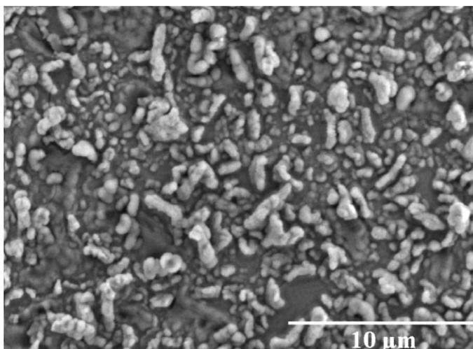
Fig. 1. SEM image of a film deposited during 4 h with the following deposition parameters:  $P_T = 50$  Pa,  $\Phi_{\text{Cr}} = 1$  sccm,  $\Phi_{\text{O}_2} = 1$  sccm,  $\Phi_{\text{Ar}} = 50$  sccm and  $F = 75$  mJ cm<sup>-2</sup>.
